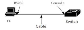
The second step to start the terminal emulation software on the PC (such as: Windows HyperTerminal) can be configured for the switch, monitoring and other operations. The cable is supplied with the host. The terminal serial port communication parameters can be set as right: rate -115200bps, eight bits data bit, one stop bit, no parity bit, no flow control. The communication parameters of HyperTerminal are configured as follows:
